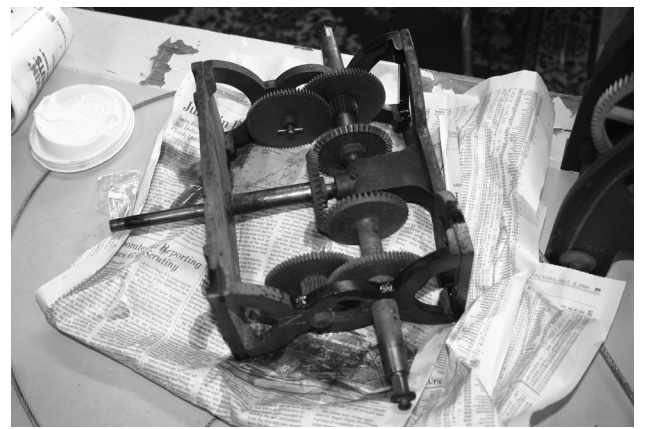
The century-old clockworks are being cleaned and greased in the basement of Dick Diefenbach's Danville home.
