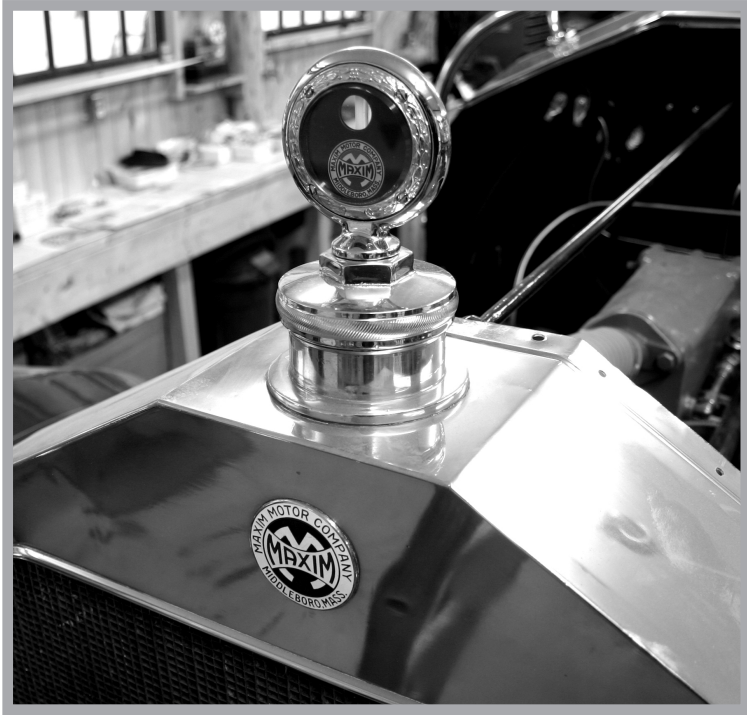
The Maxim radiator cap included a thermometer visible to the driver as a means to monitoring the temperature of the engine under the hood panels.
