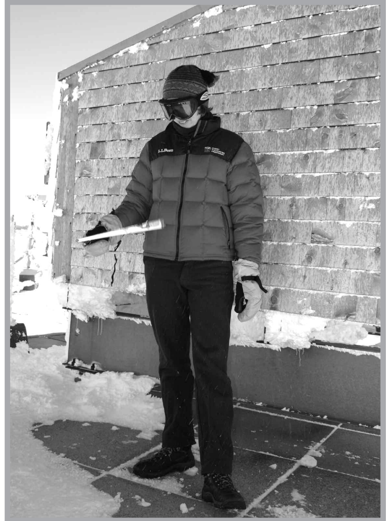
Krysia Scorko is a recent graduate of Vassar College. Working as an intern for the Mount Washington Observatory she measures relative humidity with a sling psychrometer comparing the differences between a wet bulb and a dry bulb thermometer.
